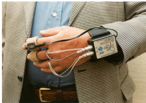
Fig. 2. The patients were recorded with polysomnography and parallel non-invasive continuous blood pressure using a Portapres device. The Portapres device is demonstrated in this foto. With two finger cuffs continuous blood pressure is recorded. The sensing cuff switches every 30 minutes and gives the other finger time to relax. The measurement principle is based on a volume clamp technique.
