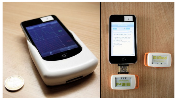
Fig. 4 Prototypes of management devices in two variants: integrated into a smartphone cover (left) and as Eventlogger with adapter for smartphone connection (right). On the left, the application for vital parameter visualization is running.
