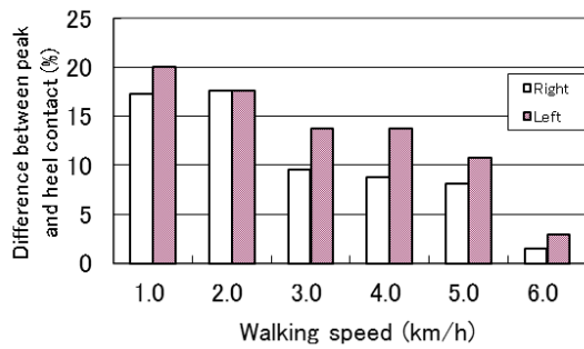
Fig. 5 Difference between peaks of the pelvis lateral translation and the heel contacts ( \Delta t )
