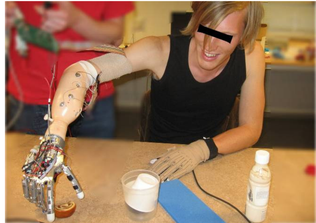
Fig. 1 Amputee reaching an object wearing the SmartHand. The unnatural reaching posture of the arm caused by the lack of the three degrees of freedom of the wrist/forearm is clear from this picture.
