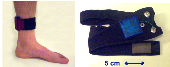
Fig. 1. (left) Photograph of wireless ankle sensor band; (right) photograph of wireless ECG sensor mounted on chest strap.
