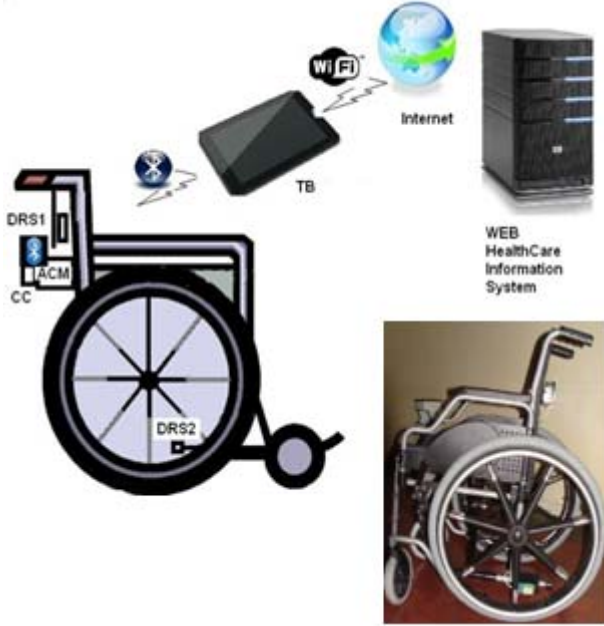
Fig. 1. System architecture based on a smart wheelchair (CC – conditioning circuit, DRS1, DRS2 - Doppler radar sensors, ACM – acquisition and communication module, TB-tablet computer).
