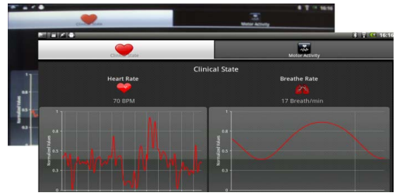
Fig. 7. The developed cardiac, respiratory and motor activity graphical interface implemented on the Android OS Tablet computer
