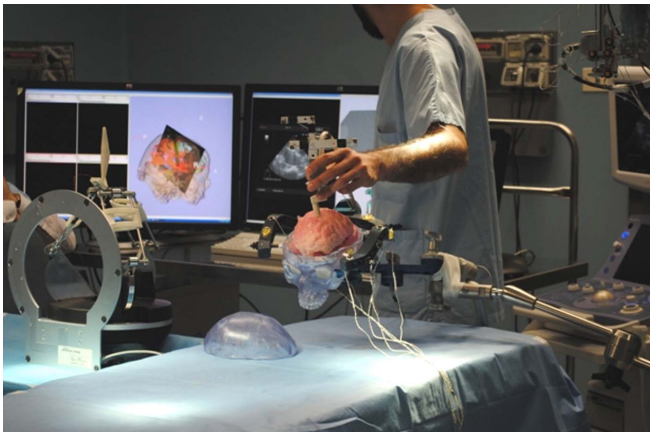
Fig. 4. Intra-operative ultrasound navigation during the ROBOCAST final demo at Ospedale Maggiore, Verona - Italy. Optical tracking of the US probe allows for visualization of the image plane in the 3D scene.
