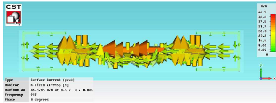
Fig. 6 Current distribution on the tag antenna
