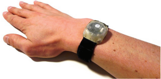
Fig. 1. ReSense sensor module in a rapid prototyped housing. Thanks to the small form factor it can easily be worn like a watch. The weight of this configuration is 21 g.
