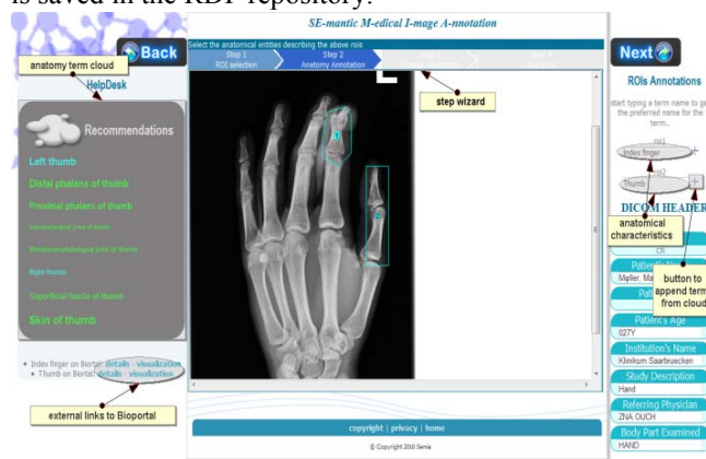
Fig. 4. Annotation procedure. : Upon loading a DICOM image, DICOM Header Tags are automatically extracted and presented to the user, who is able to edit them. In every step, the user's actions are guided through a help desk, situated on the left of the image. Apart from the guidelines, online help contains components aiming to help the user, such as the Body Region Visualization , the Anatomical Term Cloud , the Disease Ontology Tree and the terms' External Links to reference page in Bioportal. Each component appears in the appropriate step. Anatomical Term Cloud and Disease Ontology Tree are used to present the "semantic neighborhood" of the selected term in order to make meaningful recommendations regarding the anatomical and disease annotations, respectively.
