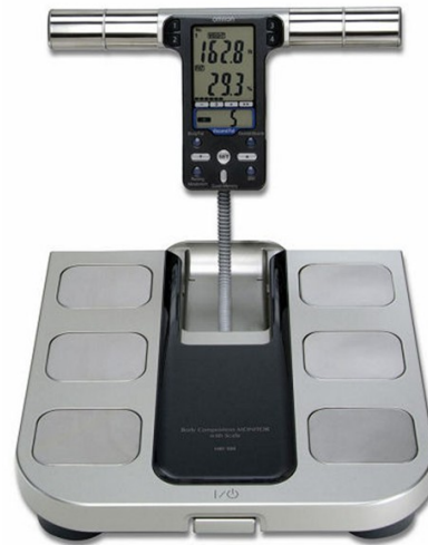
Fig. 1. A photo of the Omron HBF-500 scale used for this study. The handlebar electrodes provide two contacts for the hands that were used for ECG acquisition. The footpad electrodes were used for lower-body IPG and EMG acquisition. The cost of the scale in 2010 is approximately $80.00. (Source of photo: www.amazon.com).
