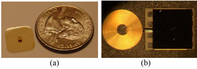
Fig. 4. (a) Optical image of the IOP sensor compared with a US quarter; (b) a photomicrograph of backside view of the IOP sensor
