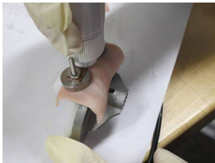
Fig. 10. Reading the RFID tag through pig skin.
