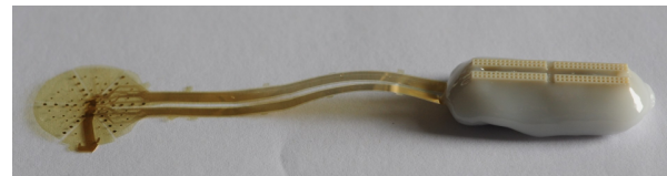
Fig. 6. The released ECoG array ready for implantation. Its reference electrode is flipped and glued to the array backside. 4 OMNETICS connectors are glued to the rigid soldering area and they are surrounded by an insulating glue.
