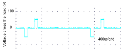
Fig. 7: This picture shows the waveform of the H-bridge output voltage across the load resistor. In the picture, the stimulator generates a train of bipolar stimulation with the parameters as follow: the stimulation current is 50mA, the stimulation duration is 50 \mu s, the stimulation frequency is 1kHz, and delay time is 100 \mu s.
