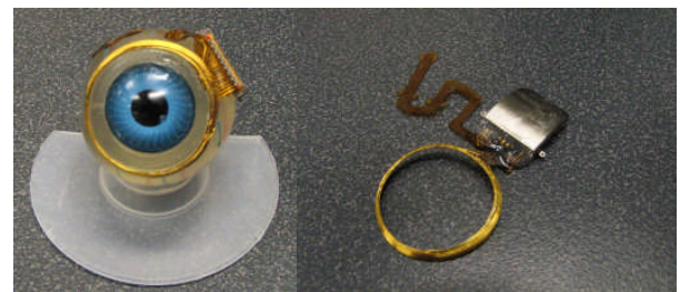
Fig. 2. Second-generation hermetically-packaged 16-channel Boston retinal prosthesis.
