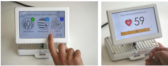
Fig. 4 The Central Telemedicine Platform. Left picture: The main menu with icons of the implemented Plug-Ins. Right picture: Pulse measurement with the integrated sensor.
