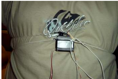
Fig. 3. Modified servo motor attached to the chest – motor placed right on sternum.
