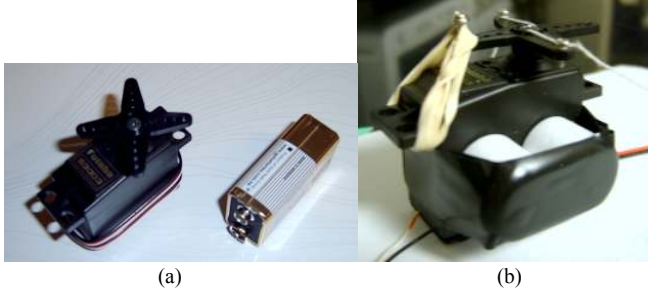
Fig. 2. Original (a) and modified wearable servo motor (b).
