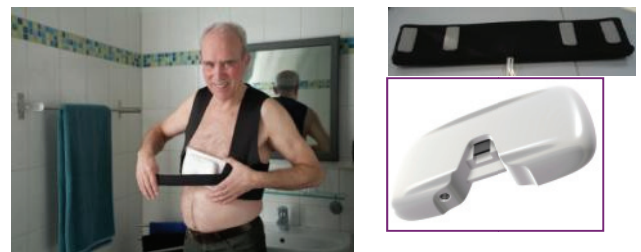
Fig. 3. The first version of the vest composed of a belt with four textile electrodes that can be adjusted to the vest and the bio-impedance device connected to the belt [4]
