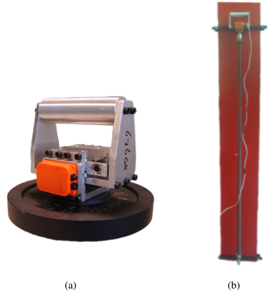
Fig. 2. Experimental setup with a mass (a) and spring (b) load. Visible is the inertial/magnetic sensor unit (orange) and force transducer embedded by load and handle.
