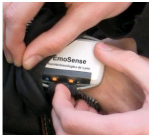
Fig. 2. EmoSense, a wrist-worn device to monitor cardiac frequency, electrodermal activity and skin temperature
