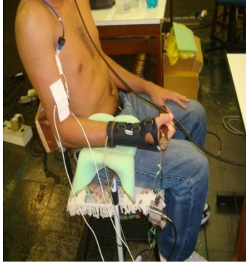
Figure 3. Subject wearing the fist orthosis, the wood hand device fixed to the cell load, the flexible linear array of electrodes, and the SiC electrodes used for the NMES.
