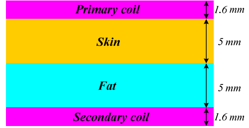
Fig. 5 Cross section of printed spiral coil with subcutaneous tissue
