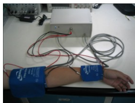
Fig. 4. The completed system hardware. Four band electrodes are attached to the subject's arm underneath the blood pressure cuffs..
