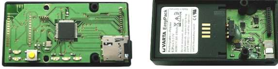
Fig. 1 - Tri-axial accelerometer based sensor (size 78x40x20 mm, weight 30g). The sensor consists of; a single liPo battery capacity 610mAh, a LIS3LV02 tri-axial accelerometer from ST Microelectronics Inc. and dsPIC (Microchip Technology Inc.) microcontroller. The Accelerometer data was downloaded via the Bluetooth link using a custom designed PC-based data logging software written in LabVIEW 2 . Calibration of the tri-axial accelerometer signals was performed using the method outlined by Ferraris et al. [10]. Signals were recorded at a frequency of 120Hz.
