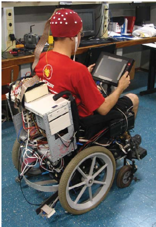
Fig. 6. Using the SSVEP-BCI to command a robotic wheelchair.
