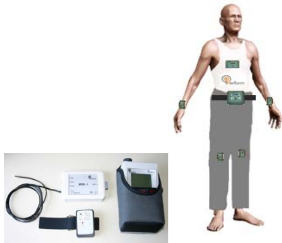
Figure 3. PERFORM System prototype including accelerometers, gyroscope and data logger (left) System placement on the body (right)
