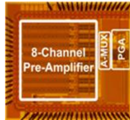
Fig.4. Die photograph of the proposed AFE.
