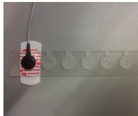
Fig 2b: Probe showing trial positions for electrode insertion with ECG electrode inserted. (2cm between adjacent positions)
