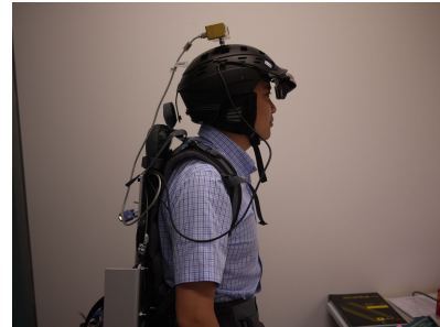
Fig. 1. Our visual processing system for extracting salient obstacles in images. On top of the helmet is a camera that captures videos that are processed by a laptop on the backpack. The results are visualized using the Emagin z800 head mounted display.
