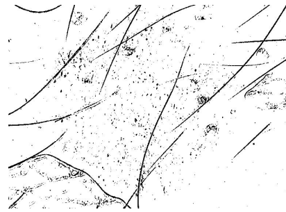
Fig. 3. Raw mask M as computed in 3 and 4 by thresholding the modified top-hat operator. Small spurious hairs are detected, while long hairs are heavily fragmented.
