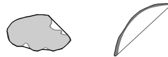
Fig. 4. Region on the left has a high D value since A \approx A_c . The region on the right, on the opposite, has a very low D value since A \ll A_c . Long and curved hairs such as the one on the right are thus easily identified.
