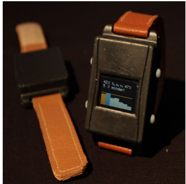
Fig. 1 The Us'em system consisting of a wristband device with accelerometer and communication modules and a watch-like device equipped with a graphical display as well (right).
