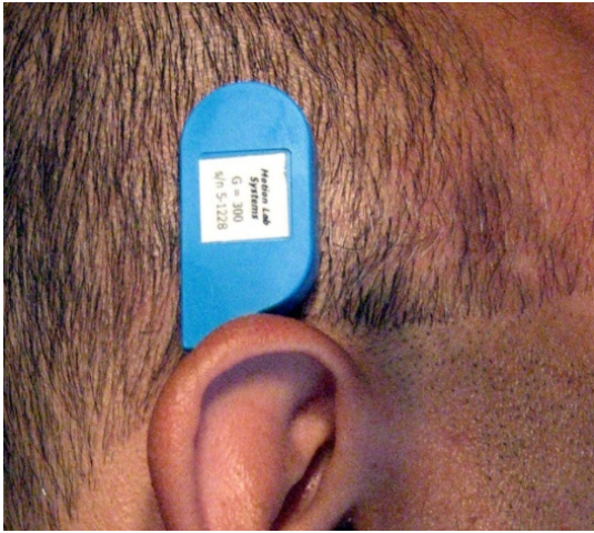
Fig. 5. Motion Lab Systems' Z03-000 sEMG sensor placed on the Auricularis superior muscle. (For visualization only.)
