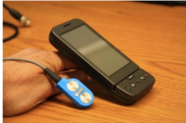
Fig. 6. Motion Lab Systems' Z03-000 sEMG sensor and Android-based HTC Dream cell phone.
