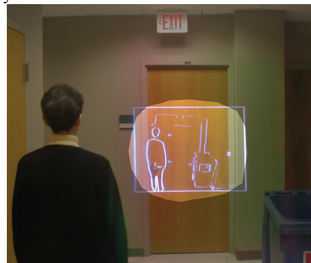
Figure 1. The augmented-vision field expander superimposes a minified outline of the ambient scene over the wearer's see-through natural vision. This is a picture taken behind the device. The highlighted area represents a typical field of view of patients with tunnel vision. With such a device a patient should be able to maintain central resolution while detecting objects outside his/her residual visual field.
