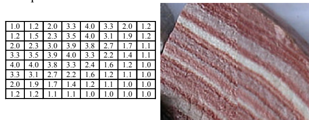
Figure 9. The mid frequency bands in the JPEG quantization table are boosted directly in the JPEG decoder (shown as scale coefficients larger than 1). The resultant enhancement is shown on the left side of the image.
