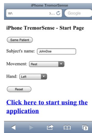
Fig. 1. A screenshot of the website, as shown on the iPhone. The user can optionally fill in their name, the type of movement they want to execute and specify the hand used (left or right). When the site is visited, a php session is created to access the on-board hardware and collect data. Each time a measurement is completed, the user is redirected back to this page.
