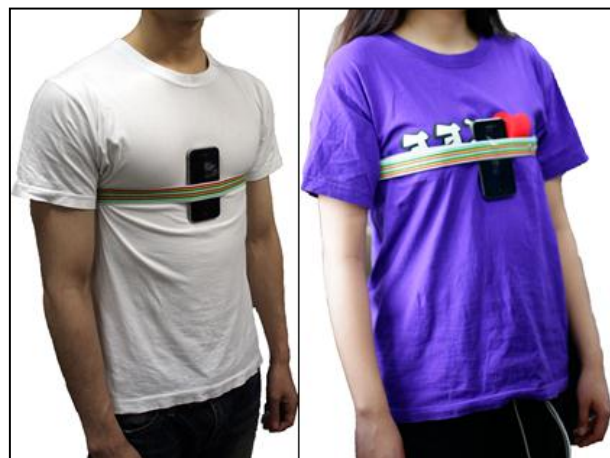
Figure 3. Heart rate extracting using iPhone accelerometer
