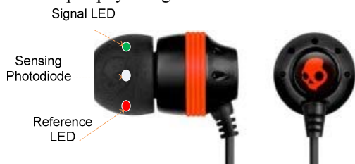
Fig 6 A typical Opto-physiological assessment sensor A novel non-invasive sensors design and set-up based on opto-physiological modeling as shown in Fig 6, is being
