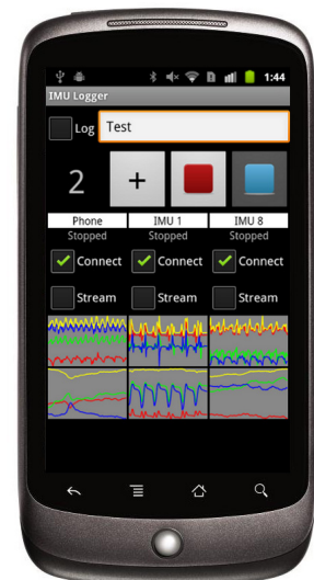
Fig 2. IMU Logger application showing three-axis accelerometer and magnetometer data from the phone and two IMUs.
