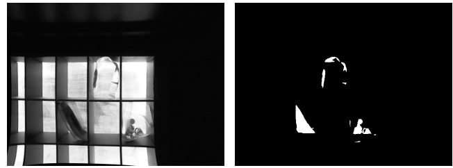
(a) Captured Gray-Scale Image (b) Subtracted Binary Image Fig. 4: A result of the background subtraction method. The white pixels in the subtracted binary image represent the presence of objects.
