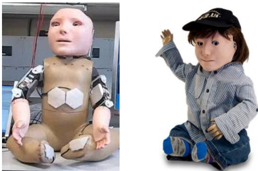
Figure 3 The robot Kaspar. The figure on the left shows the 'undressed' version revealing the tactile skin patches 1 .
