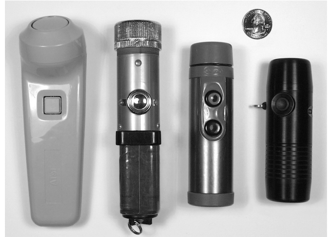
Figure 1. Examples of electrolarynx (EL) devices. From left to right: the Western Electric, Neovox, Servox, and TruTone ELs. Note the difference in size between the two older models on the left (1950s) versus the two models on the right sold today. Quarter provides size reference.
