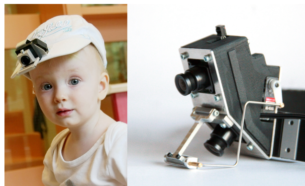
Fig. 1. Left : The WearCam worn by a typically developing 14 months old girl, fixed on a cap. Right : Closeup of the WearCam, with the two cameras and motor-controlled mirror.
