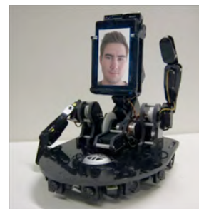
Fig. 2. The MeBot tele-presence robot. See [21].
