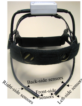
Fig. 3. eTDS-Headset prototype; the figure shows the alignment of four magneto-resistive sensors which was used in EMI cancellation.
