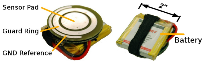
Figure 2. OLAM bottom view of sensor pad (Left). OLAM top view with battery (Right).
