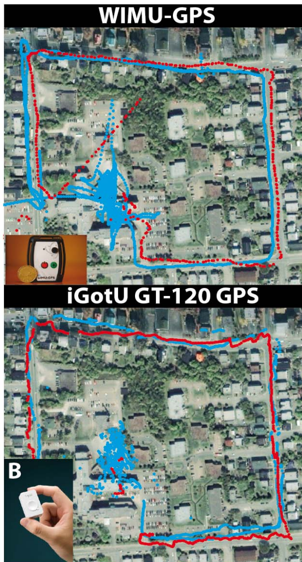
Figure 5. Trajectory comparison of the two GPS systems with the best (blue) TTFF and the worst (red).
