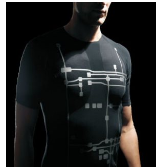
Fig. 1. The Vital Jacket is a wearable vital sign monitoring device. Due to its design in form of a light T-shirt it allows to record a one lead ECG with a sampling frequency of 200 Hz without restricting the freedom to move.
