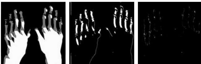
Fig. 4. Performing the CNN operation of blur, subtraction (BW and grey level) and XOR on the image.
