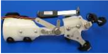
Figure 3 – prefabricated hand orthotic fitted with linear actuator for control of finger position
