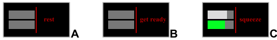
Fig. 2. To inform the subject about the current condition, visual feedback and instructions were provided over video-goggles. A: instruction to rest. B: instruction to prepare. C: Instruction to perform the motor task, i.e. pinching the right index finger and thumb to match the applied force (shown in the upper gray bar) with the reference force (shown in the lower green bar).
